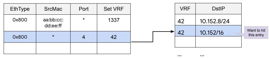
VRF == 42 & DstIP[32:16] == "10.152" & !(VRF == 42 & DstIP[32:8] == "10.152.8") & !(...) // encode VRF assignment
