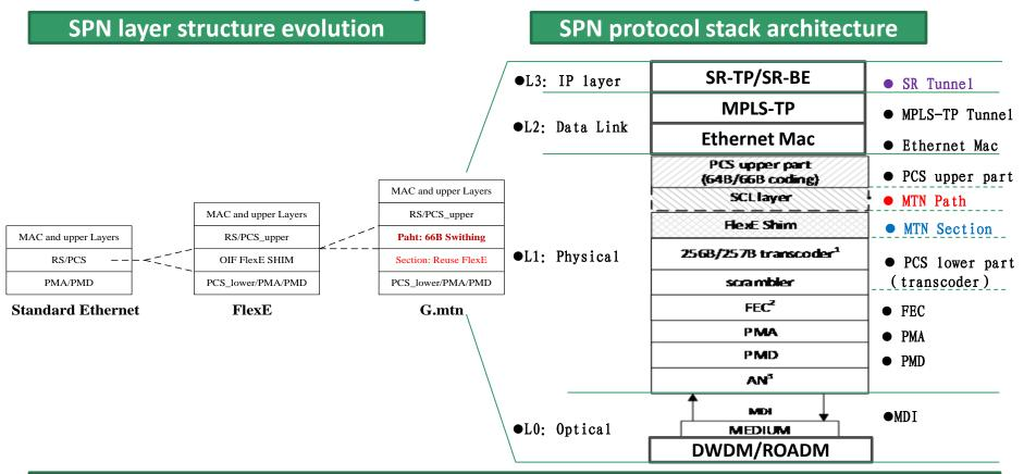
SPN innovatively introduces SPN channel layer, integrates TDM and packet switching, and integrates L0 layer to L3 layer into an organic whole.
