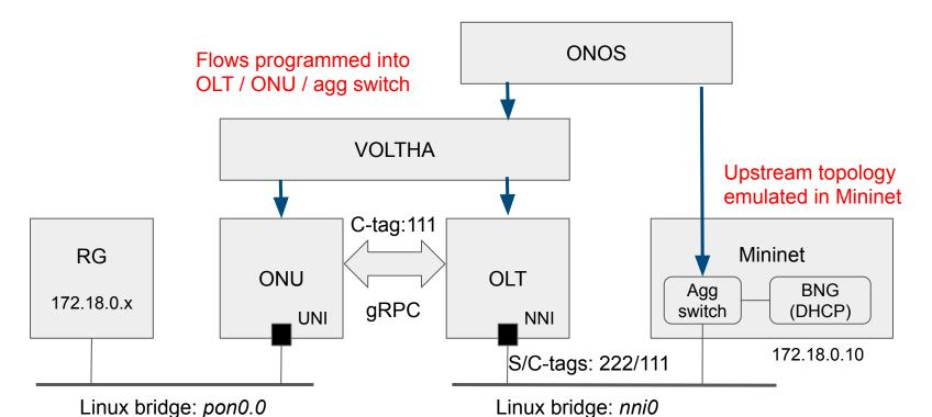
Linux bridges for Ethernet (L2) connectivity btw components
